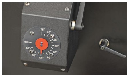
Precise bevel angle adjustment
