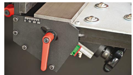
Simple setting of bevel width
